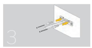
Fix the support in its definitive position with The other two wall plugs and screws to avoid the shelf displacing the levelled position.
