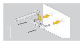
Place the support on the wall with the supplied wall plugs and screws and place the rod on the support.
