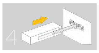
Finally, place the shelf in position. This can subsequently be removed whenever necessary to carry out further adjustments.
