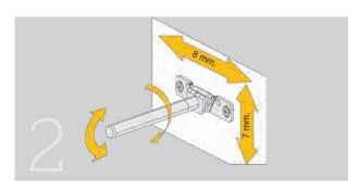
Oval holes allow accurate levelling. It can be horizontally adjusted by moving the rod along the support. Furthermore, the gradient may easily be adjusted by just turning the rod.
